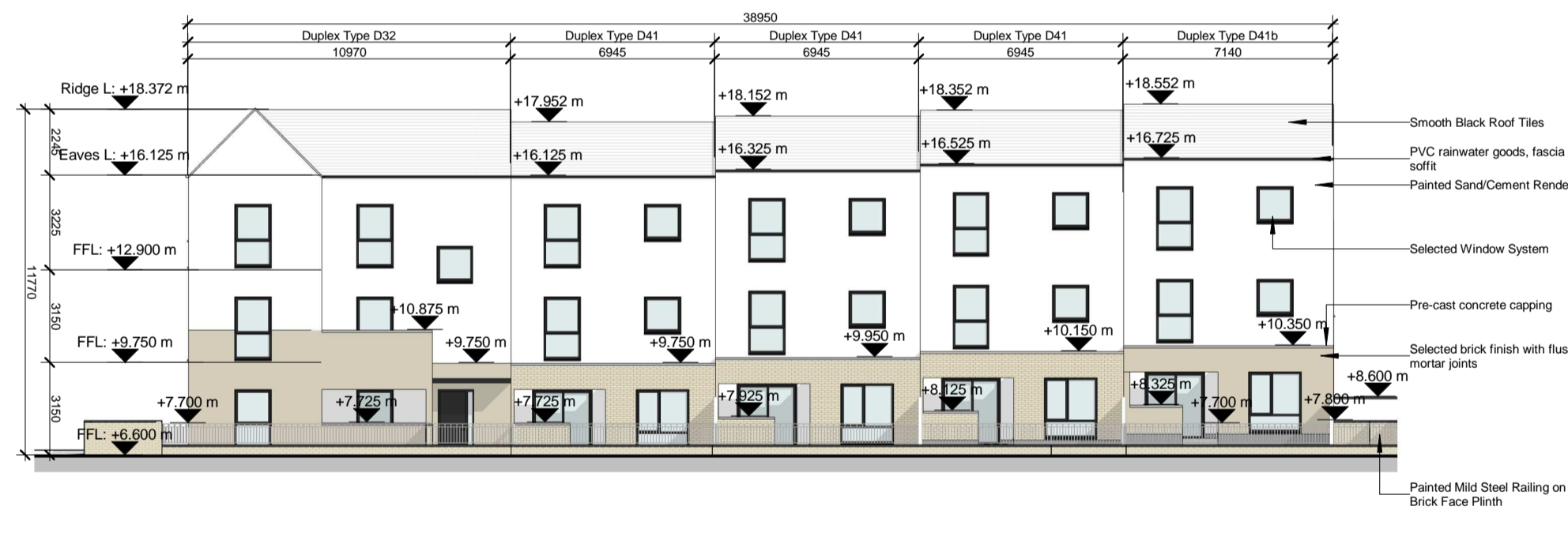
6 Duplex Block E East (Rear) Elevation 1 : 200
